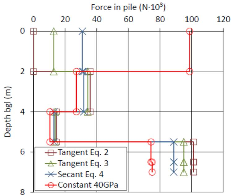
Fig. 6 Unit skin friction distribution at ultimate state for pile T7B
