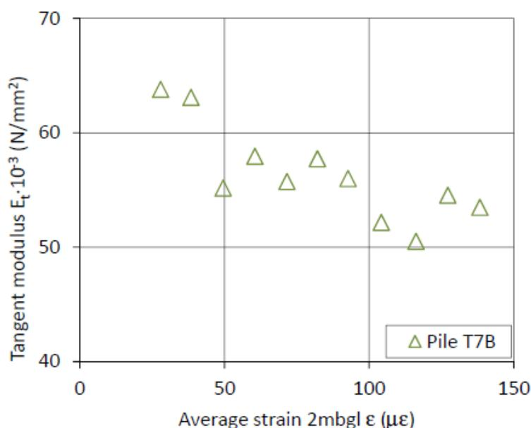
**Fig. 4** Tangent modulus plot for gages 2mbgl in pile T7B
