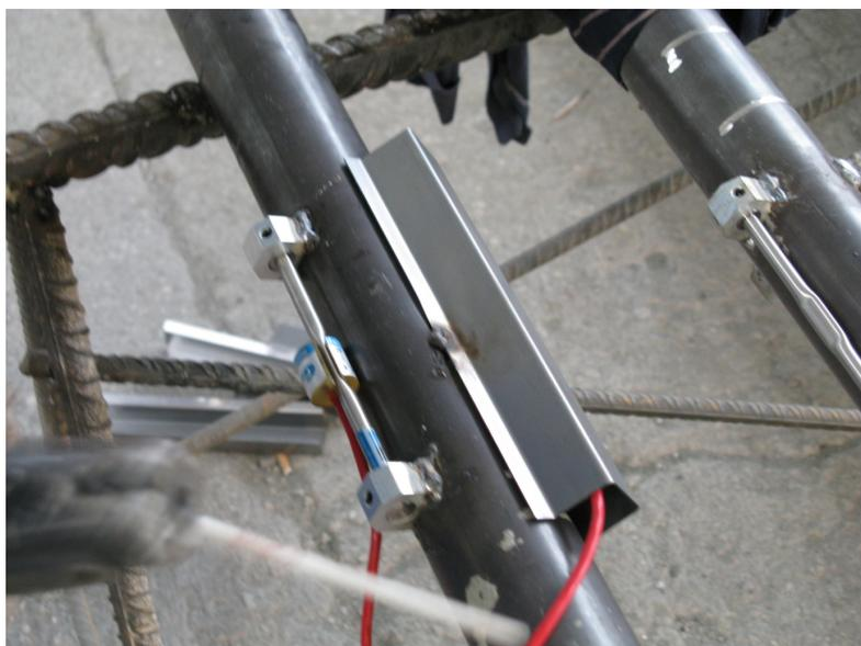
*Fig. 1 Strain gages and cover assembly*
