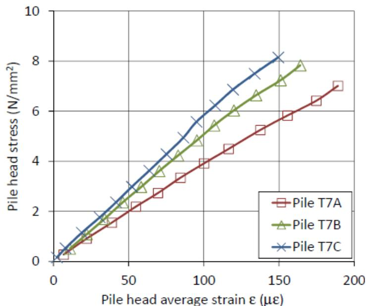
Fig. 3 Stress-strain relationship for T7 piles at the first gage level
