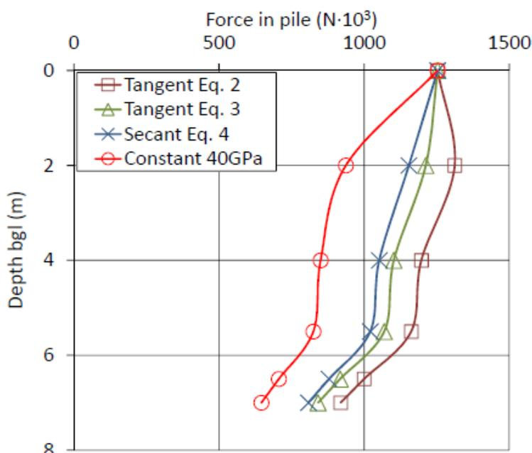
Fig. 5 Force distribution at ultimate state for pile T7B
