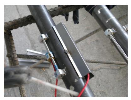
Fig. 1 Strain gages and cover assembly
