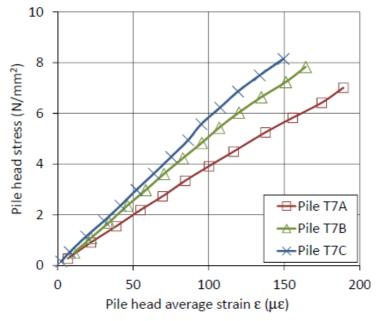
Fig. 3 Stress-strain relationship for T7 piles at the first gage level
